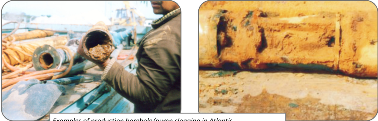
Examples of production borehole/pump clogging in Atlantis.
